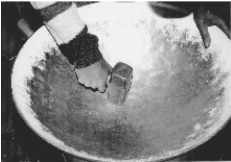
Fig. 2.13 Smoothing the sink with the backing hammer.
