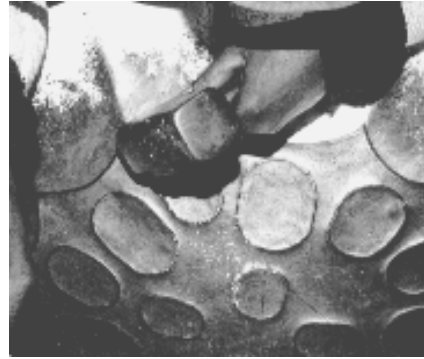
Fig. 5.9 Levelling of the radial border of outer notes before grooving.
