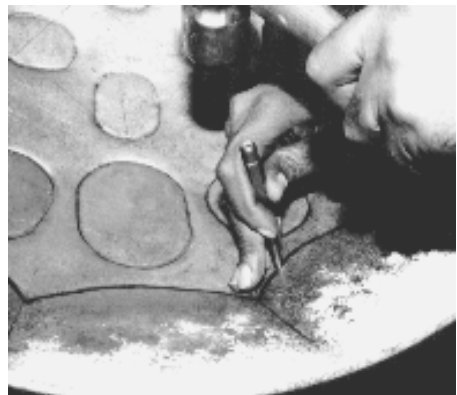
Fig. 5.8 Grooving the inner border of an outer note.
