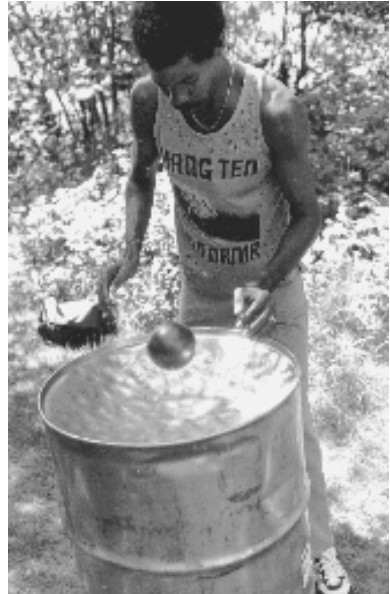
Fig. 2.5 Sinking with a shot-put. Photograph by Linus Torell.
