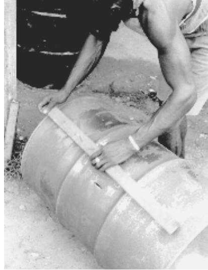
Fig. 7.1 Marking the drum for cutting.
