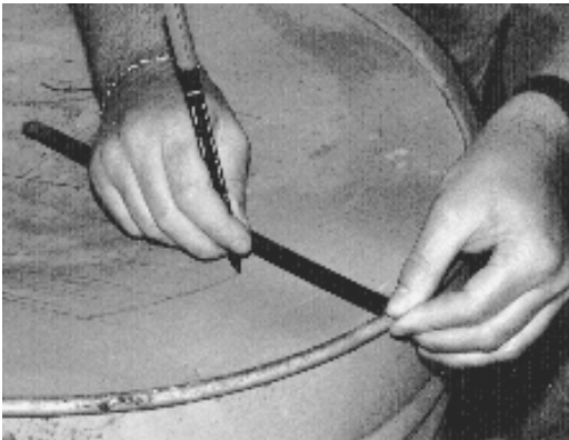
Fig. 2.4 Method to make concentric circles.
