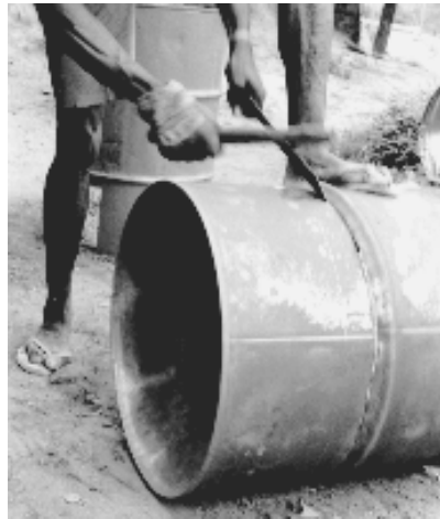
Fig. 7.2 Cutting the drum with a cutlass.
