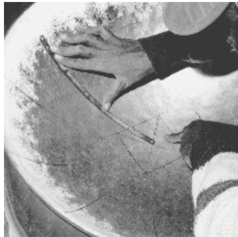
Fig. 3.3 Drawing the radial lines of the outer notes. Note the centre marking.
