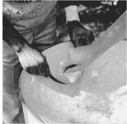
Fig. 3.5 Marking the curved inner border of an outer note with a bent ruler.
