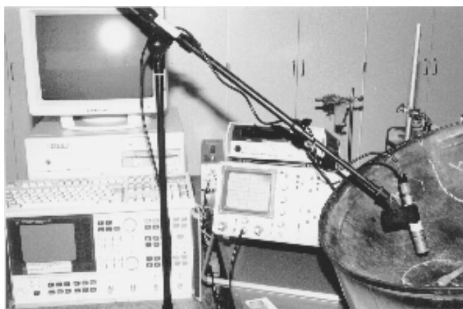
Fig. 20.1 Research on the steel pan. Experimental setup with (left to right) frequency analyser, computer, oscilloscope, frequency counter and microphone.
