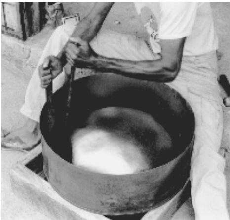
Fig. 9.5 Raising an outer note with a "crowbar" iron. Note the cutlass blade held against the side of the drum as protection.
