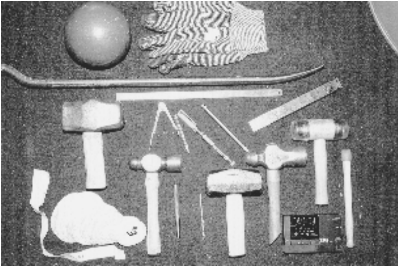
Fig. B.1 Main part of the tools needed for panmaking.
