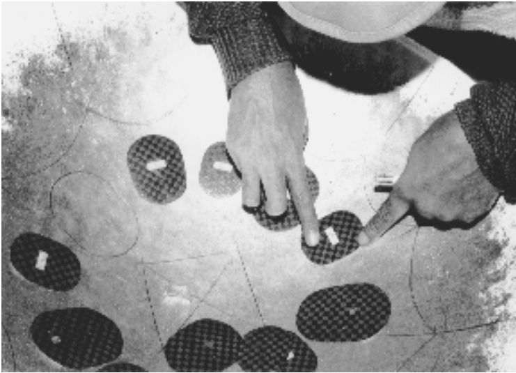
Fig. 3.6 Spread out the templates of all the inner notes to check space and positioning before marking.
