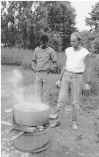
Fig. 8.3 Burning the pan, using the left-over part of the drum as a fireplace.
