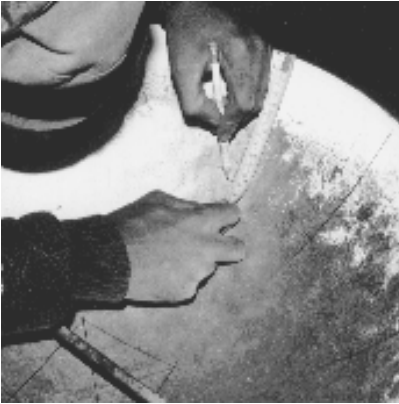
Fig. 3.4 Marking the length of the radial groove of the outer notes.
