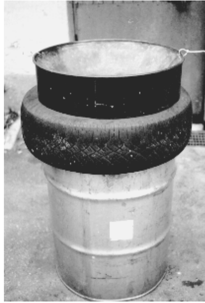
Fig. 9.4 Temporary tuning stand made from the left-over part of the drum and a car tyre.
